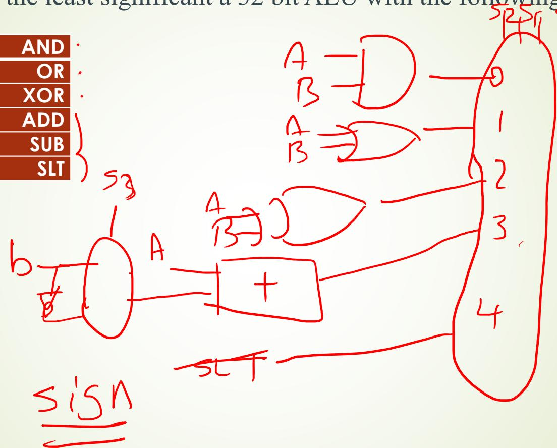
4. Design the most significant a 32 bit ALU with the following functionality.
